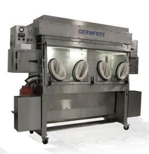
The LFGI Series provides either positive or negative pressure HEPA-filtered unidirectional (laminar) airflow for patient, personnel, and product protection. The unit can be configured for positive (non-hazardous) or negative (hazardous) pressure to comply with USP <797> and NIOSH recommendations.
