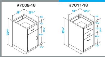
This example shows **PHICE AB** model # 7002-18 reconfigured to a non **PHICE AB** model # 7011-18, The cupboard door is removed and replaced by a second 7<sup>1</sup>/<sub>4</sub>" box drawer and one bulk storage drawer with the new drawer slides provided.
