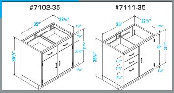
This example shows **MILLE AB** model # 7102-35 reconfigured to a non **MILLE AB** model # 7111-35. The left hand door is removed and replaced by a second 7" letter drawer and one bulk storage drawer. The three quarter height door is removed and replaced by one full height door.
